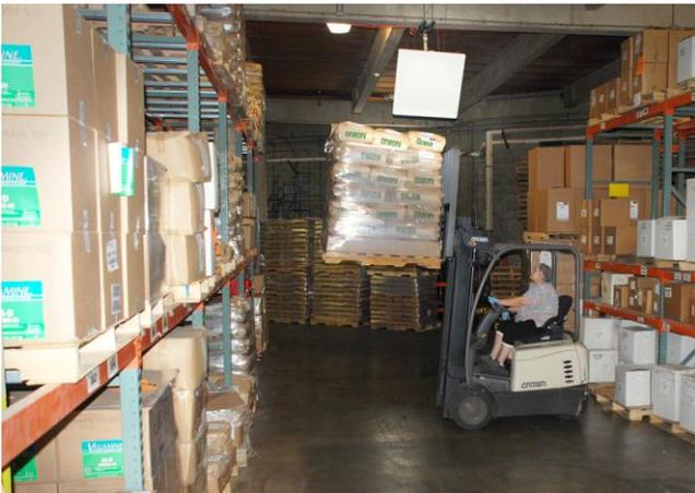
With an RF Controls smart antenna, seen here directly over the pallet, companies can track RFID-tagged items automatically as they move around the warehouse.
